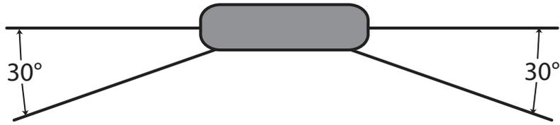
Required angle of pull for test - 30° from horizontal in the vertical direction
