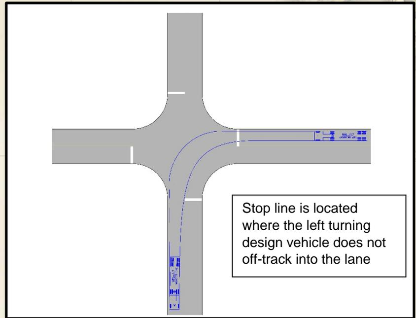
FIGURE 4: Stop Line Versus Design Vehicle Example
