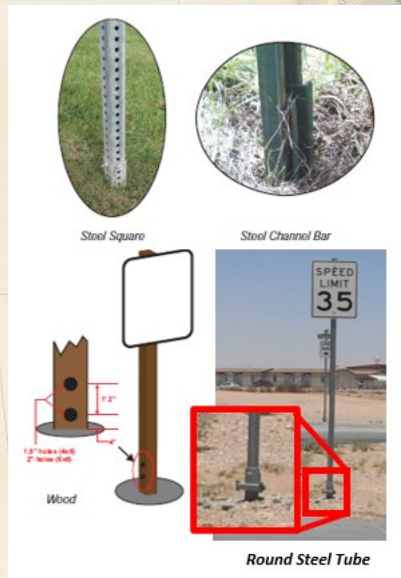
Common Breakaway Sign Posts
