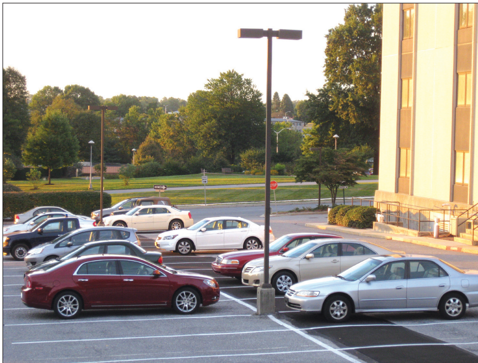
Exhibit 21.8: Parking Lot Lighting using Full Cutoff Lamps
