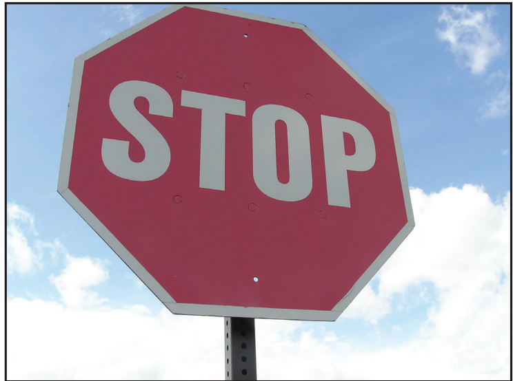
Exhibit 7.10: An Unacceptable, Non-retroreflective Sign
