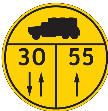
Bidirectional, Dual Classification MLC sign
