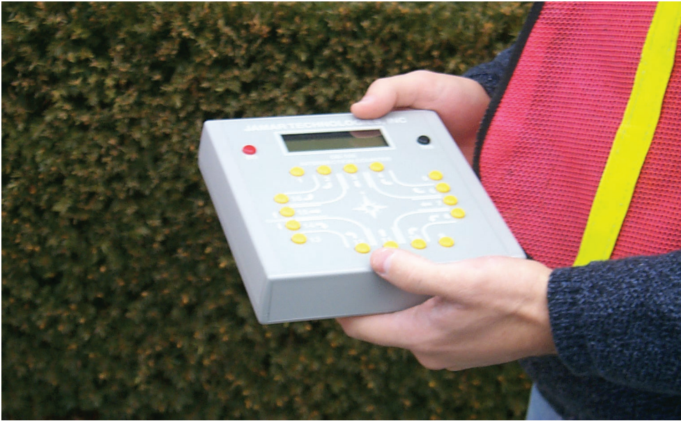
Exhibit 1.1: Typical Turning Movement Counter
